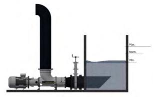
Figure 2.22 Example of dry set-up for a main water pump Source: Lykkegaard.
