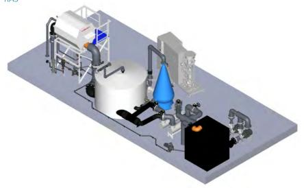
Water is filtered in a mechanical filter on left side before ozonation in a chamber at center. Water passes through two UV systems and finally enters the black holding tank.
