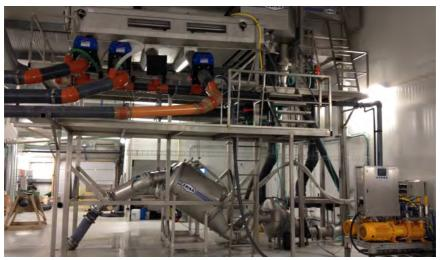
The fish are graded into different size categories before they are counted using infrared light and returned to the tanks by gravity.
