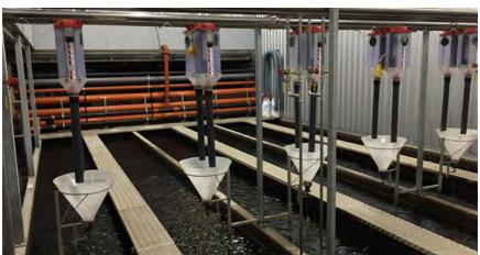
Figure 5.9 An example of an automated feeding system
