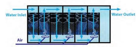
Both types of biofilters can be used in the same system, using the moving bed filter to avoid the trouble of back-washing, and the fixed bed to benefit from the effect of microparticle removal. Thus, there are several solutions for the final design of biofilter systems depending on farm size, species to be cultured, fish sizes, etc.
